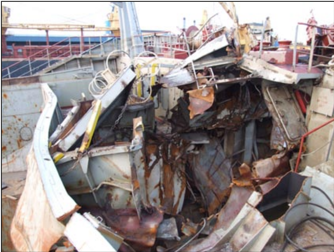
Damage to fore'sle head
