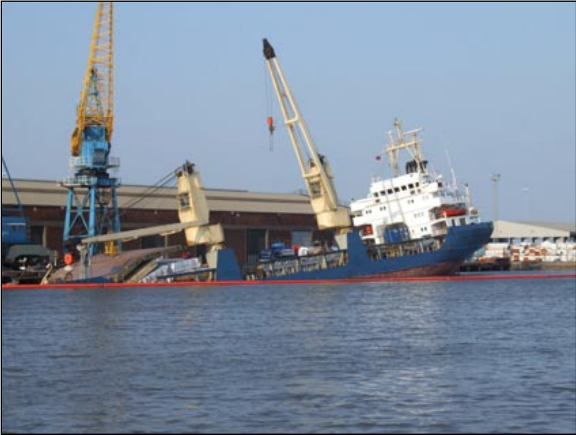
Skagern's bow settled on dock bottom
